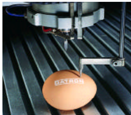
Mapping surfaces and finding features with the Z-axis probe from Datron takes about 1.5 sec per point. Rather than fitting in the spindle, the probe sits on a pneumatically driven arm that unfolds to make measurements. Tool changes are unnecessary
