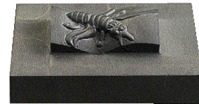
The latest generation of high-speed hard milling centers excels at cutting graphite. A Digma 300 from Hansco cut this electrode in 43.5 min with maximum speeds and feeds of 35,000 rpm and 118 ipm
