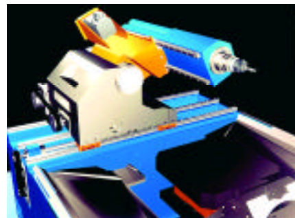
The Bobcat from Lamb Technicon exploits hybrid kinematics to accelerate at 1.5 g. Two high-pitch ballscrews lying parallel in the direction of the X axis generate all movement throughout the X-Y plane. They move the spindle and its carrier both in an arc and in a line. The resulting kinematic advantage multiplies velocity and acceleration
