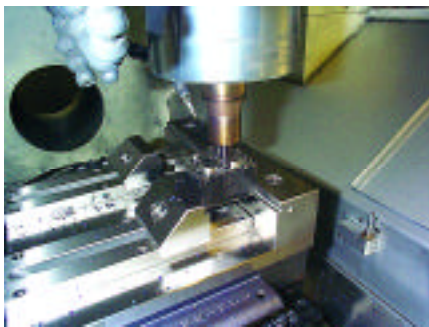
As roughing in this test piece proves, 42,000-rpm spindles can be stout enough for cutting a Rc 50 tool steel that is similar to H13. The 10-mm tool is spinning at 9000 rpm on a Roeders RFM600 machining center and traveling at 120 ipm in a 0.025-in. cut
