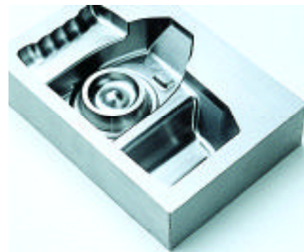
No hardening and less time in polishing on an EDM are the advantages of milling mold cavities on high-speed hard-milling centers. This cavity was cut from prehardened steel on the Vibra-Free machining center from Compumachine
