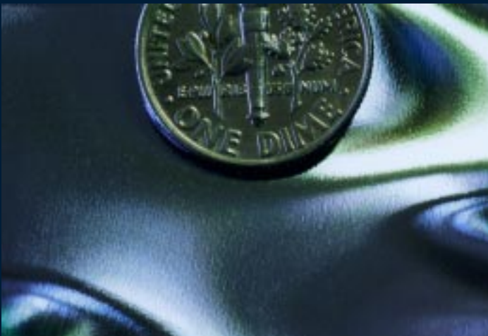
Wavy Surface, 420 Stainless Steel, HRC54
