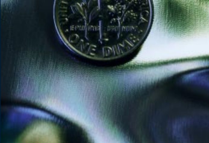
Wavy Surface, 420 Stainless Steel, HRC54
