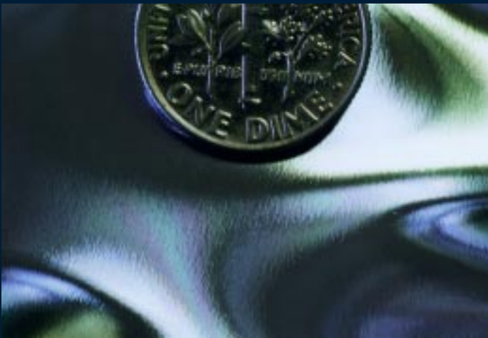
Wavy Surface, 420 Stainless Steel, HRC54
